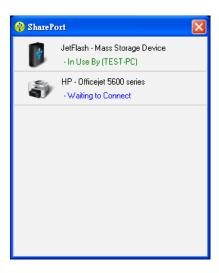
Move the cursor to Use By (Owner) and click on Disconnect to virtually disconnect the USB device.
