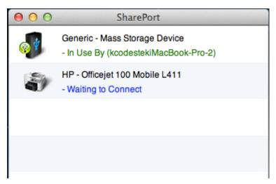
You can then move the cursor to In Use By (Owner) and click Disconnect to virtually disconnect the USB device.
