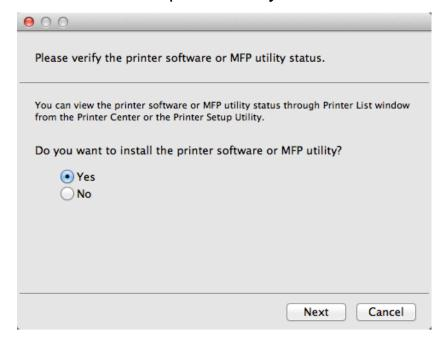
■ Insert the CD-ROM of the multifunction printer and follow the instructions to install the multifunction printer's driver. When the installation process prompts you to connect the multifunction printer to your Mac, click **Next**.
