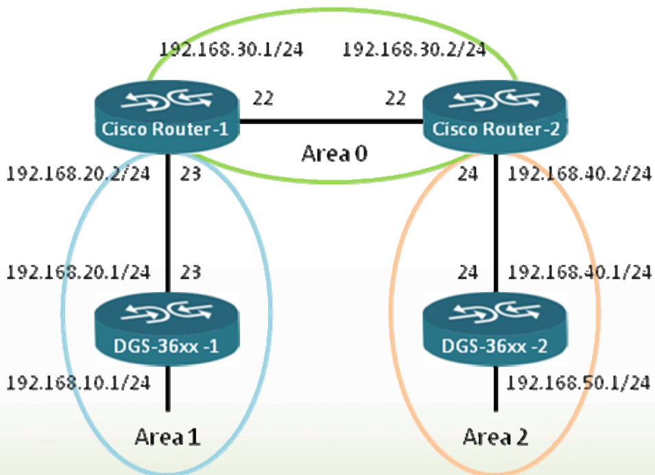
Figure-6 Multiple OSPF Areas Configuration
