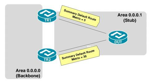
There are two OSPF areas (0.0.0.0, 0.0.0.1) in this topology. TR1 and TR2 are Area Border Router which generate default route carried in Type 3 Summary LSA into Stub area 0.0.0.1. Both of them send default route with different metric value. DUT will use best metric (smallest) of default route.
