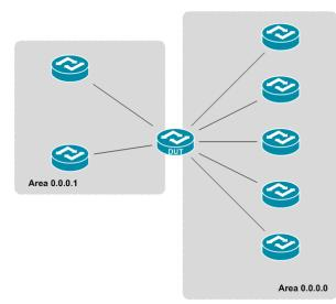
There are two OSPF area (0.0.0.0 and 0.0.0.1) in this topology, the DUT is an area border router which attach to both of area.
