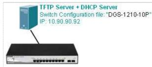
**Note:** DGS-1210 support DHCP Auto Configuration function at firmware R2, so please make sure your DUT upgrade to the latest firmware version
